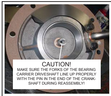
Fig. 5-5 Driveshaft Alignment
