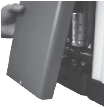
REMOVE FRONT FASCIA PANEL BY TILTING OUTWARDS AND DOWNWARDS.
