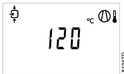
Shut-down screen, element outlet temperature
