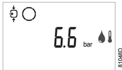
Main screen with the dewpoint temperature warning
