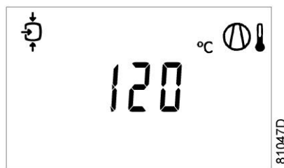
Shut-down screen, element outlet temperature
