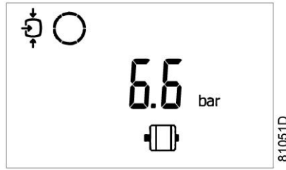
Main screen with shut-down indication, motor overload
