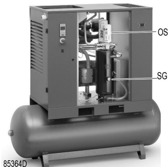
Oil level sight-glass
